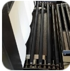
High Density Rollers - Close Roller Spacing 1/2" Gap
