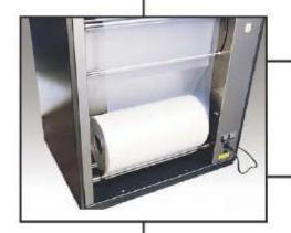
Film roll sets on powered film unwind rollers and feeds toward front of machine. Uses single-wound polyethylene sheeting, plain or random printed. Maximum film thickness 2 mill. Finished bag meets USPS regulations if using postal approved polyethylene.
