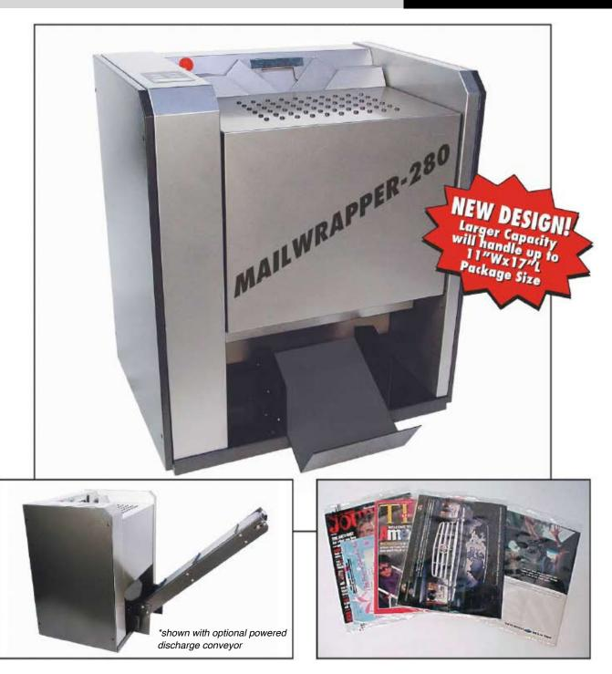
The Mailwrapper-280 is the low cost alternative to high speed magazine poly bagging. Great for magazines, periodicals, instruction booklets or loose sheets of paper. An operator simply inserts one or several magazines up to 1/2" thick into the adjustable width forming plow. The poly film is automatically wrapped around the product and is discharges into catch tray or optional powered discharge conveyor.
