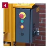
**1** Compact your recyclables and eject the bale with a two-handed operation. **2** Move the bales and store until collection. **3** The flexible tying system allow you to use either plastic strapping or metal wire. **4** A full bale light indicates when the baler has reached full capacity.
