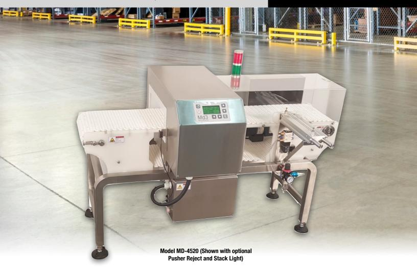
The **Hawk Series of Metal Detectors** is designed for easy integration into food production lines. Superior levels of metal detection sensitivity are attained using multi-frequency sensor engine technology. With the "Auto Learn" feature the Hawk Series are easy to set up and operate with the lowest cost of ownership.
