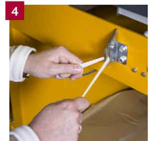
**1** Eject the finished bale after compacting waste. **2** Remove and store finished bale until pickup. **3** Using the safe two-hand ejection system, the finished bale is ejected automatically. **4** Knife mounted on front of baler allows safe cutting of straps.
