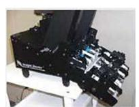
The R-12/20B feeders include a separate start photo sensor that can be mounted on your packaging line to trigger the feeder at exactly the right time.
